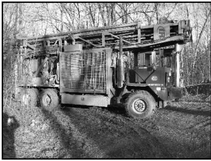
Drill rig used to tap groundwater
