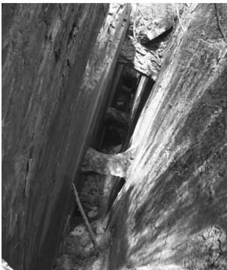
FIG. 9—Photograph looking north into an abandoned cement mine in the Rosendale Member of the Rondout Formation (see also Fig. 7) in the west-dipping limb of the Hickory Bush anticline near the Fourth Binnewater Lake (Fig. 1). This mine was completed in strata that are dipping at roughly 80^\circ from horizontal. Pillars are approximately 4-m (13-ft) tall.
